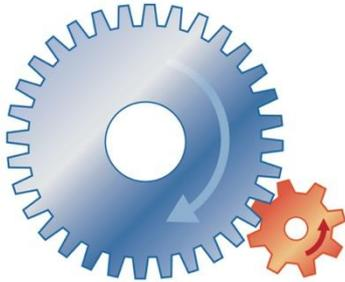
It takes four times as much force to turn the large wheel once as it does to turn the small wheel once.
