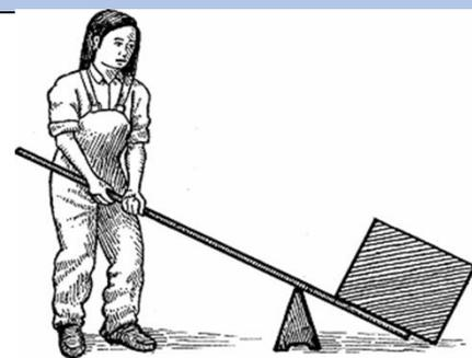
A **lever** is a rigid arm that is braced against a turning point, or **fulcrum**. Pushing at one end of the arm creates a force at the other end.
